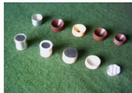
Floats for fuel gauge made with syntactic foam
