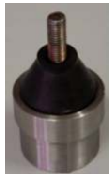
Vibration mount based on magnetorheological fluid
