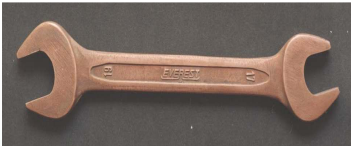
Photograph of the Non-sparking tool (Spanner) made of Cu-4.5Ti alloy
