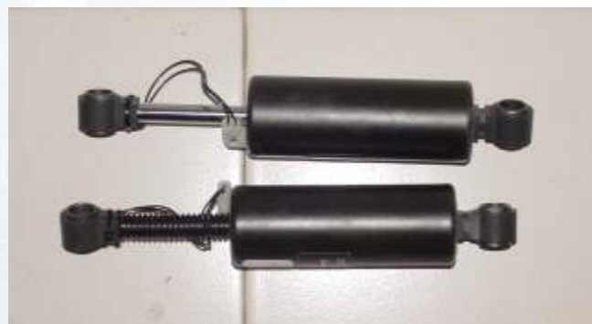
Damper based on magnetorheological fluid
